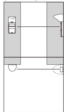
\* The sensor and reflector units should be installed uprightly and vertically. Make sure that the reflector's front side faces the sensor as illustrated.
