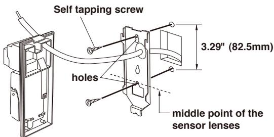
Pull the wire through the sensor body (back to front) and attach it to the terminals on the sensor.
