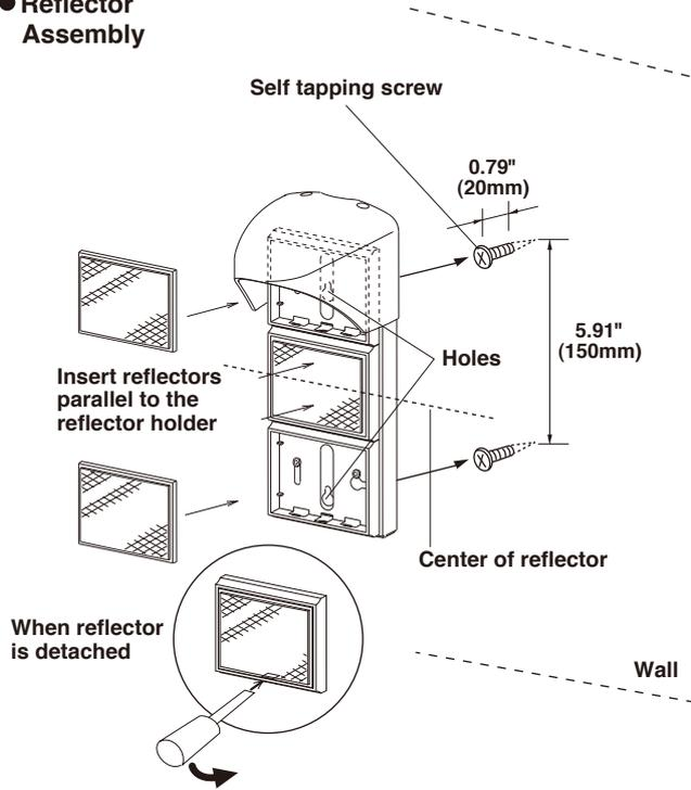
① Insert self tapping screws into the wall by about 0.79" (20mm) and hang the reflector unit back plate on them using the holes.
