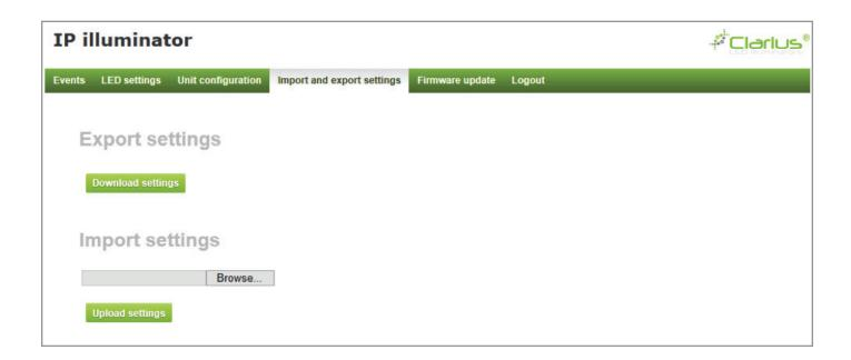
The user can export settings from a given illuminator by clicking on the download settings button as shown above and saving the settings as a CFG file. The user can then import this file into another illuminator by selecting browse next to the import settings section as shown above and then simply click Upload settings.
