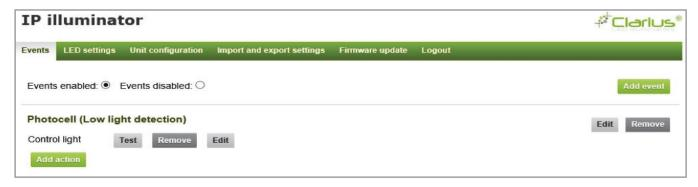
The Photocell (Low light detection) event as shown above is pre-programmed into the illuminator, however, this too can be removed by the user if desired by clicking remove on the right-hand side of the screen.
