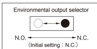
The environmental signal is initiated if the beam reception level is reduced by poor weather conditions (dense fog or torrential rain etc.).
