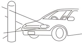
● Avoid strong light from the sun, automobile headlights etc. shining on transmitter and receiver directly. (Avoid light within  $\pm 2^\circ$  degrees of optical axis.)
