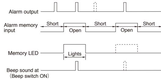
Connect / disconnect terminal ① and ⊕ terminal (① or ②)
