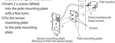
⑤Follow the same procedure as wall mounting (from③) for wiring.
