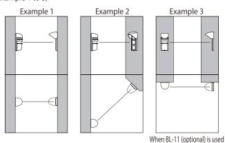
Install the reflector directly, facing the front of the optical unit as much as possible.
