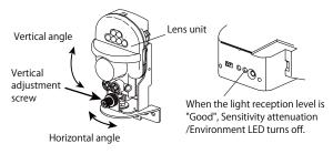
When the direction of the optical axis roughly matches the reflector, a beep sound begins which changes according to the light reception level as below.
