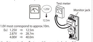
(3) If the distance to the reflector and the converted value of the test meter do not match, fine adjust the optical axis of the lens unit or remove any objects near to the protection line.
