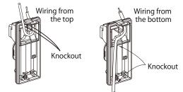
⑤After wiring is completed, adjust alignment, attach cover and check operation.
