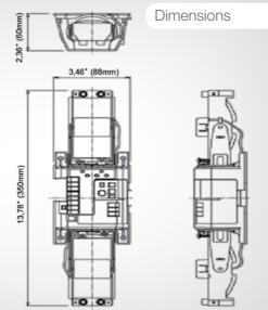
Available to cover up to 200m, this infrared beam feature a unique Double Modulated Beam signal making them extremely resistant to both direct and reflected sunlight up to 50,000 lux.
